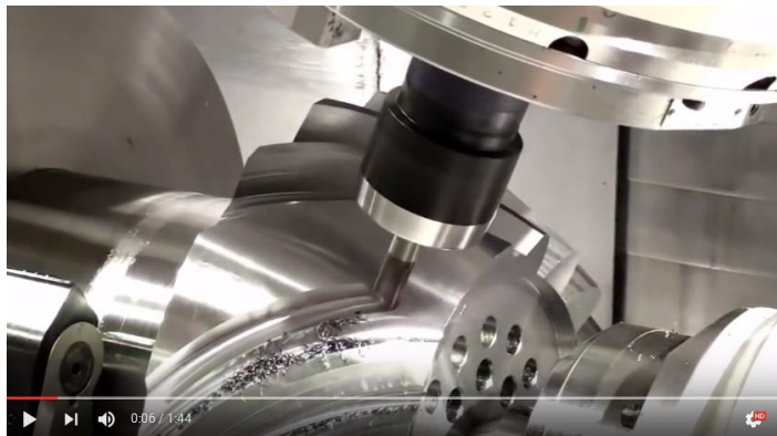
Super modern machine CNC 5 axis in machining spiral bevel gear, MAZAK INTEGREX e-670H-II
